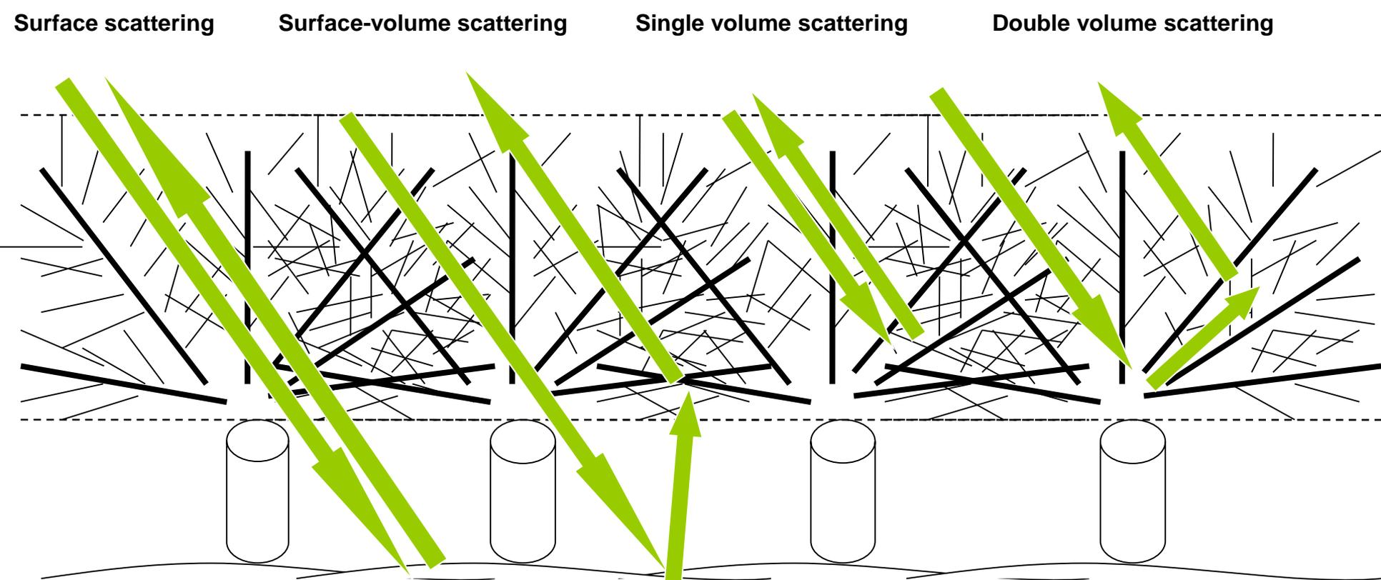
*Backscattering components based on the iterative solutions of the radiative transfer equations*
