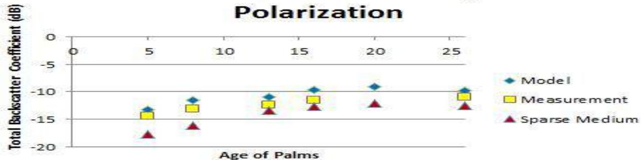
**(b) Total Backscatter Coefficient, Model VS Measured Data, VV Polarization**
