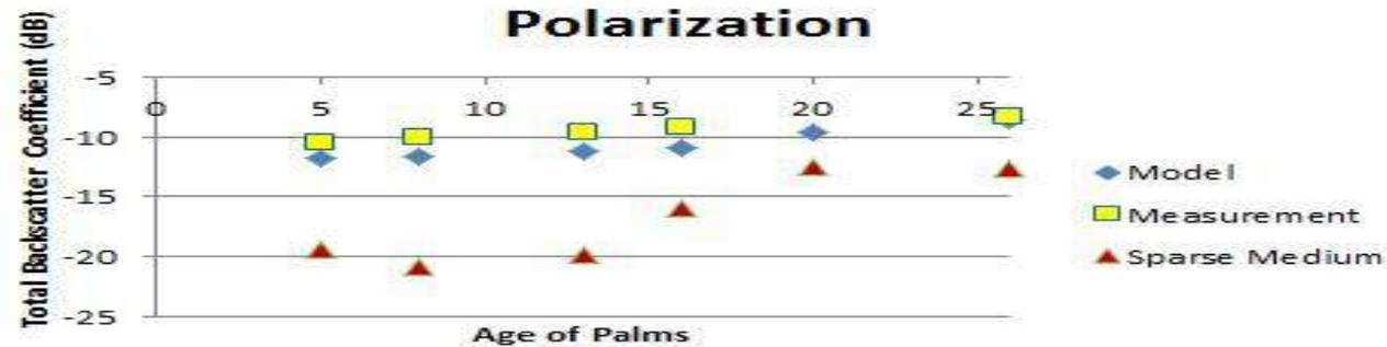
**(c) Total Backscatter Coefficient, Model VS Measured Data, HV Polarization**
